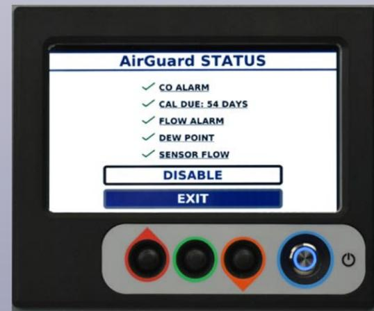
From the main display selecting the check function, AirGuard will report “System Status” indicating any faults, CO and differential dew point status, last calibration date, respiratory flow, and sensor flow measurement.
