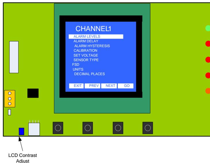
**Figure 4: LC-8 Display Contrast Adjustment**
