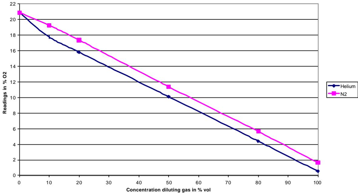
For Sensor type B, note the much more accurate readings from the oxygen sensor in the presence of helium. Note also that the readings for Helium are slightly below expected values, a failure in the safe direction. Nitrogen diluent causes readings only slightly above the theoretical values.
