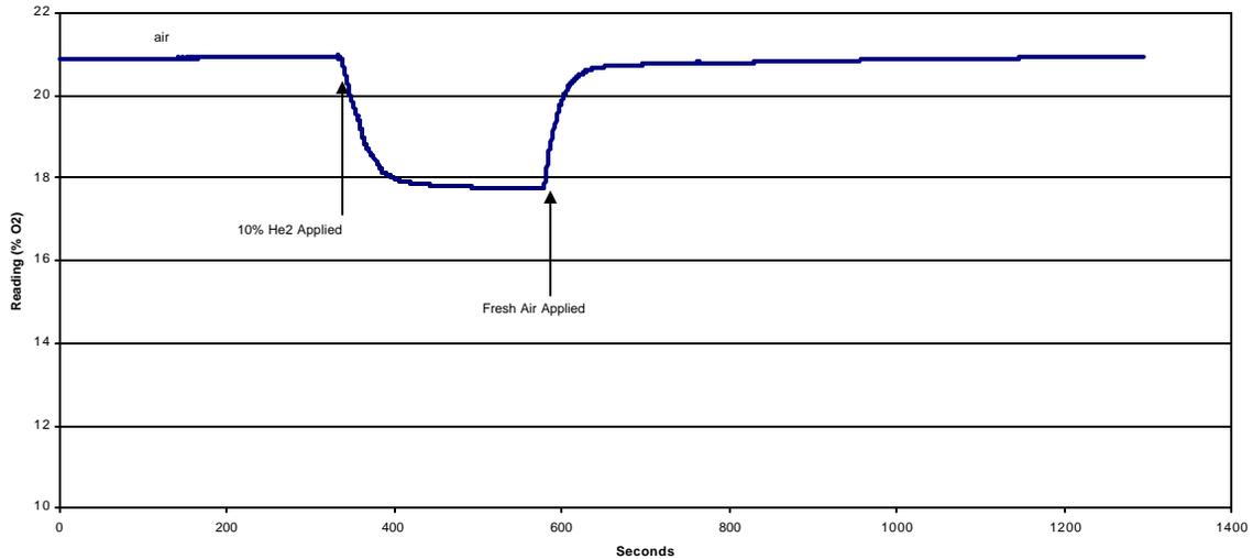
The step change response to 10% Helium and back to fresh air is normal for the Sensor Type B.
