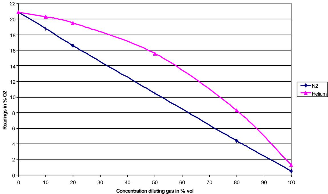
Note that the sensor readings show a false positive concentration of oxygen when the background gas is Helium. When Nitrogen is background gas, the readings are very close to the theoretical values in the table below.
