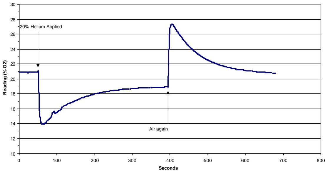
In the previous graph, note the quick initial responses to the Helium shown as decreased O<sub>2</sub> readings, followed by upward drift to a false “safe” condition. Once the Helium is removed, a substantial false positive over-recovery, then drift down towards proper levels.
