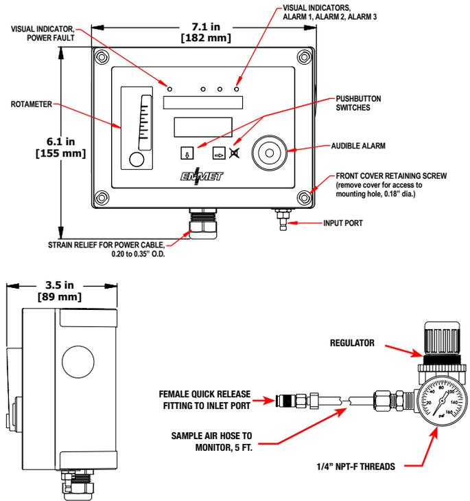
CO-GUARD is supplied with a regulator and 5 foot hose for connection to the monitor. Connection from the facility air supply to the regulator is 1/4 inch NPT female.
