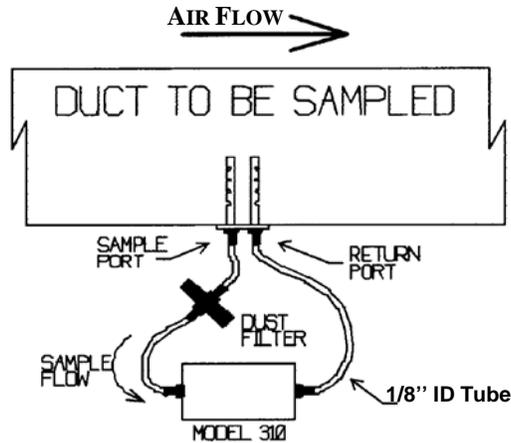
Figure 3: Duct Sampling Schematic
