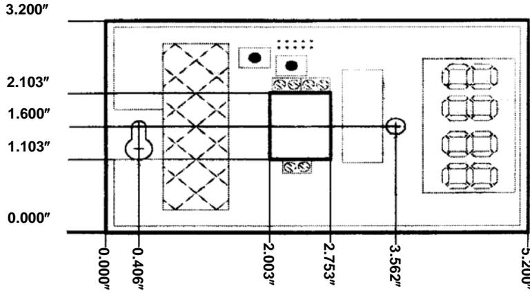
Figure 1: CD-1300 Series, Mounting Dimensions
